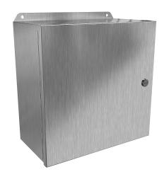
Hammond Eclipse Junior series enclosure, NEMA 3R/4/4X/12/13,  $12 \times 12 \times 6$  in (HxWxD), wall mount, 316 stainless steel, #4 brush finish, single-door, 1/4-turn semi-flush 316 stainless steel latch.
