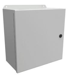
Hammond Eclipse Junior series enclosure, NEMA 3R/4/12/13, 12 x 12 x 6in (HxWxD), wall mount, carbon steel, RAL 7035 light gray, powder coat finish, single-door, 1/4-turn semi-flush latch.
