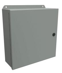
Hammond Eclipse Junior series enclosure, NEMA 3R/4/12/13,  $12 \times 12 \times 4in$  (HxWxD), wall mount, carbon steel, ANSI 61 gray, powder coat finish, single-door, 1/4-turn semi-flush latch.
