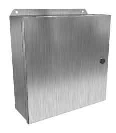
Hammond Eclipse Junior series enclosure, NEMA 3R/4/4X/12/13,  $12 \times 12 \times 4$  in (HxWxD), wall mount, 304 stainless steel, #4 brush finish, single-door, 1/4-turn semi-flush 316 stainless steel latch.
