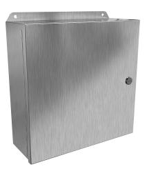
Hammond Eclipse Junior series enclosure, NEMA 3R/4/4X/12/13, 12 x 12 x 4in (HxWxD), wall mount, 316 stainless steel, #4 brush finish, single-door, 1/4-turn semi-flush 316 stainless steel latch.
