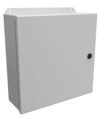
Hammond Eclipse Junior series enclosure, NEMA 3R/4/12/13, 12 x 12 x 4in (HxWxD), wall mount, carbon steel, RAL 7035 light gray, powder coat finish, single-door, 1/4-turn semi-flush latch.
