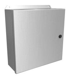
Hammond Eclipse Junior series enclosure, NEMA 3R/4/4X/12/13, 12 x 12 x 4in (HxWxD), wall mount, 5052-H32 aluminum, singledoor, 1/4-turn semi-flush 316 stainless steel latch.
