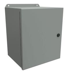
Hammond Eclipse Junior series enclosure, NEMA 3R/4/12/13,  $12 \times 10 \times 8$  in (HxWxD), wall mount, carbon steel, ANSI 61 gray, powder coat finish, single-door, 1/4-turn semi-flush latch.
