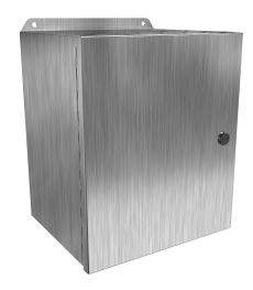
Hammond Eclipse Junior series enclosure, NEMA 3R/4/4X/12/13,  $12 \times 10 \times 8$  in (HxWxD), wall mount, 304 stainless steel, #4 brush finish, single-door, 1/4-turn semi-flush 316 stainless steel latch.
