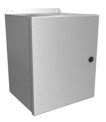
Hammond Eclipse Junior series enclosure, NEMA 3R/4/4X/12/13, 12 x 10 x 8in (HxWxD), wall mount, 5052-H32 aluminum, single-door, 1/4-turn semi-flush 316 stainless steel latch.
