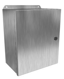
Hammond Eclipse Junior series enclosure, NEMA 3R/4/4X/12/13, 12 x 10 x 6in (HxWxD), wall mount, 304 stainless steel, #4 brush finish, single-door, 1/4-turn semi-flush 316 stainless steel latch.
