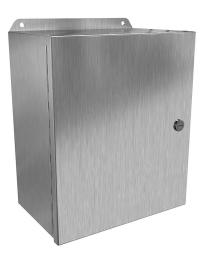
Hammond Eclipse Junior series enclosure, NEMA 3R/4/4X/12/13, 12 x 10 x 6in (HxWxD), wall mount, 316 stainless steel, #4 brush finish, single-door, 1/4-turn semi-flush 316 stainless steel latch.
