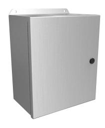
Hammond Eclipse Junior series enclosure, NEMA 3R/4/4X/12/13, 12 x 10 x 6in (HxWxD), wall mount, 5052-H32 aluminum, singledoor, 1/4-turn semi-flush 316 stainless steel latch.
