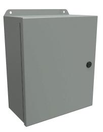
Hammond Eclipse Junior series enclosure, NEMA 3R/4/12/13,  $12 \times 10 \times 5$ in (HxWxD), wall mount, carbon steel, ANSI 61 gray, powder coat finish, single-door, 1/4-turn semi-flush latch.
