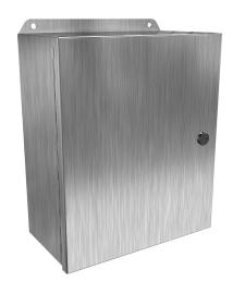
Hammond Eclipse Junior series enclosure, NEMA 3R/4/4X/12/13,  $12 \times 10 \times 5$  in (HxWxD), wall mount, 304 stainless steel, #4 brush finish, single-door, 1/4-turn semi-flush 316 stainless steel latch.
