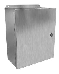
Hammond Eclipse Junior series enclosure, NEMA 3R/4/4X/12/13,  $12 \times 10 \times 5$  in (HxWxD), wall mount, 316 stainless steel, #4 brush finish, single-door, 1/4-turn semi-flush 316 stainless steel latch.
