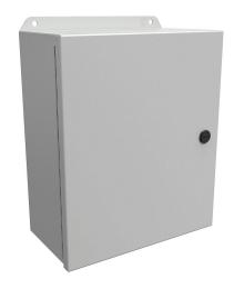
Hammond Eclipse Junior series enclosure, NEMA 3R/4/12/13,  $12 \times 10 \times 5$  in (HxWxD), wall mount, carbon steel, RAL 7035 light gray, powder coat finish, single-door, 1/4-turn semi-flush latch.
