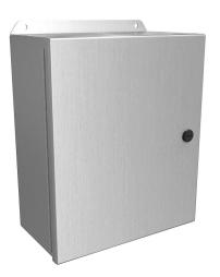
Hammond Eclipse Junior series enclosure, NEMA 3R/4/4X/12/13, 12 x 10 x 5in (HxWxD), wall mount, 5052-H32 aluminum, single-door, 1/4-turn semi-flush 316 stainless steel latch.
