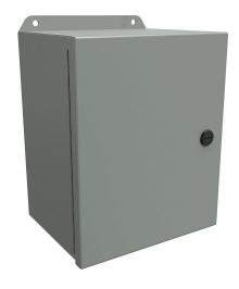
Hammond Eclipse Junior series enclosure, NEMA 3R/4/12/13,  $10 \times 8 \times 6$  in (HxWxD), wall mount, carbon steel, ANSI 61 gray, powder coat finish, single-door, 1/4-turn semi-flush latch.
