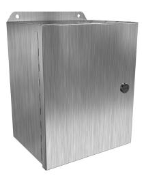
Hammond Eclipse Junior series enclosure, NEMA 3R/4/4X/12/13, 10 x 8 x 6in (HxWxD), wall mount, 304 stainless steel, #4 brush finish, single-door, 1/4-turn semi-flush 316 stainless steel latch.
