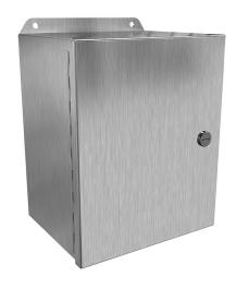
Hammond Eclipse Junior series enclosure, NEMA 3R/4/4X/12/13,  $10 \times 8 \times 6$  in (HxWxD), wall mount, 316 stainless steel, #4 brush finish, single-door, 1/4-turn semi-flush 316 stainless steel latch.
