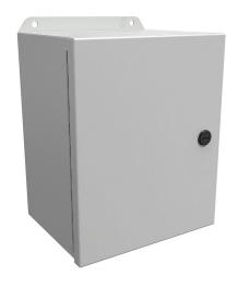
Hammond Eclipse Junior series enclosure, NEMA 3R/4/12/13,  $10 \times 8 \times 6$  in (HxWxD), wall mount, carbon steel, RAL 7035 light gray, powder coat finish, single-door, 1/4-turn semi-flush latch.
