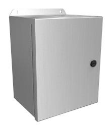
Hammond Eclipse Junior series enclosure, NEMA 3R/4/4X/12/13, 10 x 8 x 6in (HxWxD), wall mount, 5052-H32 aluminum, singledoor, 1/4-turn semi-flush 316 stainless steel latch.
