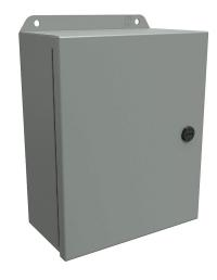
Hammond Eclipse Junior series enclosure, NEMA 3R/4/12/13,  $10 \times 8 \times 4$ in (HxWxD), wall mount, carbon steel, ANSI 61 gray, powder coat finish, single-door, 1/4-turn semi-flush latch.
