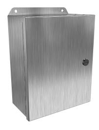
Hammond Eclipse Junior series enclosure, NEMA 3R/4/4X/12/13,  $10 \times 8 \times 4$  in (HxWxD), wall mount, 304 stainless steel, #4 brush finish, single-door, 1/4-turn semi-flush 316 stainless steel latch.
