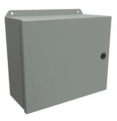
Hammond Eclipse Junior series enclosure, NEMA 3R/4/12/13, 10 x 12 x 5in (HxWxD), wall mount, carbon steel, ANSI 61 gray, powder coat finish, single-door, 1/4-turn semi-flush latch.
