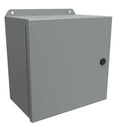
Hammond Eclipse Junior series enclosure, NEMA 3R/4/12/13,  $10 \times 10 \times 6in$  (HxWxD), wall mount, carbon steel, ANSI 61 gray, powder coat finish, single-door, 1/4-turn semi-flush latch.
