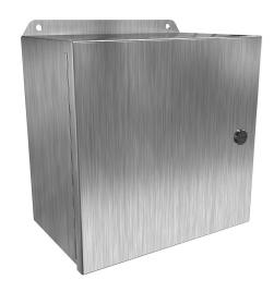
Hammond Eclipse Junior series enclosure, NEMA 3R/4/4X/12/13,  $10 \times 10 \times 6$  in (HxWxD), wall mount, 304 stainless steel, #4 brush finish, single-door, 1/4-turn semi-flush 316 stainless steel latch.
