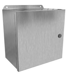
Hammond Eclipse Junior series enclosure, NEMA 3R/4/4X/12/13, 10 x 10 x 6in (HxWxD), wall mount, 316 stainless steel, #4 brush finish, single-door, 1/4-turn semi-flush 316 stainless steel latch.
