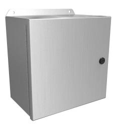
Hammond Eclipse Junior series enclosure, NEMA 3R/4/4X/12/13, 10 x 10 x 6in (HxWxD), wall mount, 5052-H32 aluminum, single-door, 1/4-turn semi-flush 316 stainless steel latch.
