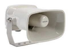
Patlite audible signal horn, 110 dB at 1m, 293 Hz to 3.5 kHz tone frequency, (32) selectable tone(s), 12-24 VDC, bracket mount, polycarbonate housing, off-white, IP65.
