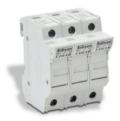
Edison modular fuse holder, accepts Class Midget fuses, 30A, 600V, 3-pole, 18-4 AWG copper only, integral pressure plate with separate spade connection, 35mm DIN rail mount. Package of 4.
