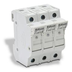
Edison modular fuse holder, with indicator, accepts Class Midget fuses, 30A, 600V, 3-pole, 18-4 AWG copper only, integral pressure plate with separate spade connection, 35mm DIN rail mount.
