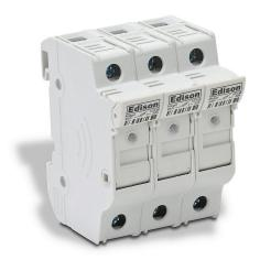
Edison modular fuse holder, with indicator, accepts Class Midget fuses, 30A, 600V, 3-pole, 18-4 AWG copper only, integral pressure plate with separate spade connection, 35mm DIN rail mount. Package of 4.
