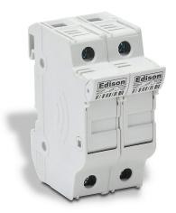
Edison modular fuse holder, accepts Class Midget fuses, 30A, 600V, 2-pole, 18-4 AWG copper only, integral pressure plate with separate spade connection, 35mm DIN rail mount.
