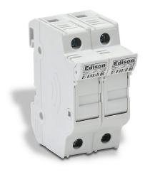
Edison modular fuse holder, accepts Class Midget fuses, 30A, 600V, 2-pole, 18-4 AWG copper only, integral pressure plate with separate spade connection, 35mm DIN rail mount. Package of 6.
