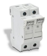
Edison modular fuse holder, with indicator, accepts Class Midget fuses, 30A, 600V, 2-pole, 18-4 AWG copper only, integral pressure plate with separate spade connection, 35mm DIN rail mount.
