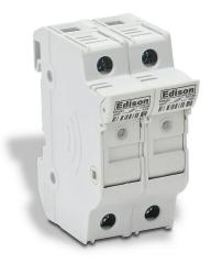
Edison modular fuse holder, with indicator, accepts Class Midget fuses, 30A, 600V, 2-pole, 18-4 AWG copper only, integral pressure plate with separate spade connection, 35mm DIN rail mount. Package of 6.
