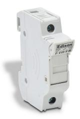
Edison modular fuse holder, accepts Class Midget fuses, 30A, 600V, 1-pole, 18-4 AWG copper only, integral pressure plate with separate spade connection, 35mm DIN rail mount.
