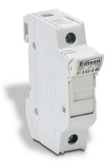
Edison modular fuse holder, accepts Class Midget fuses, 30A, 600V, 1-pole, 18-4 AWG copper only, integral pressure plate with separate spade connection, 35mm DIN rail mount. Package of 12.
