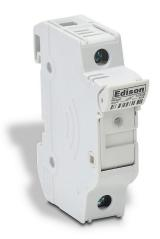
Edison modular fuse holder, with indicator, accepts Class Midget fuses, 30A, 600V, 1-pole, 18-4 AWG copper only, integral pressure plate with separate spade connection, 35mm DIN rail mount.
