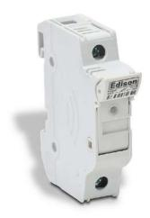
Edison modular fuse holder, with indicator, accepts Class Midget fuses, 30A, 600V, 1-pole, 18-4 AWG copper only, integral pressure plate with separate spade connection, 35mm DIN rail mount. Package of 12.
