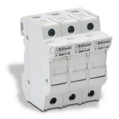
Edison modular fuse holder, accepts Class CC fuses, 30A, 600V, 3-pole, 18-4 AWG copper only, integral pressure plate with separate spade connection, 35mm DIN rail mount.
