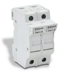
Edison modular fuse holder, accepts Class CC fuses, 30A, 600V, 2-pole, 18-4 AWG copper only, integral pressure plate with separate spade connection, 35mm DIN rail mount.
