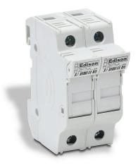
Edison modular fuse holder, accepts Class CC fuses, 30A, 600V, 2-pole, 18-4 AWG copper only, integral pressure plate with separate spade connection, 35mm DIN rail mount. Package of 6.
