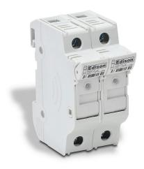
Edison modular fuse holder, with indicator, accepts Class CC fuses, 30A, 600V, 2-pole, 18-4 AWG copper only, integral pressure plate with separate spade connection, 35mm DIN rail mount.
