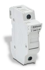
Edison modular fuse holder, accepts Class CC fuses, 30A, 600V, 1-pole, 18-4 AWG copper only, integral pressure plate with separate spade connection, 35mm DIN rail mount.
