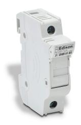
Edison modular fuse holder, accepts Class CC fuses, 30A, 600V, 1-pole, 18-4 AWG copper only, integral pressure plate with separate spade connection, 35mm DIN rail mount. Package of 12.
