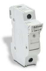
Edison modular fuse holder, with indicator, accepts Class CC fuses, 30A, 600V, 1-pole, 18-4 AWG copper only, integral pressure plate with separate spade connection, 35mm DIN rail mount.
