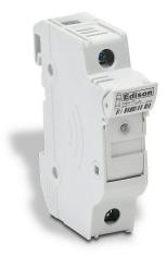
Edison modular fuse holder, with indicator, accepts Class CC fuses, 30A, 600V, 1-pole, 18-4 AWG copper only, integral pressure plate with separate spade connection, 35mm DIN rail mount. Package of 12.
